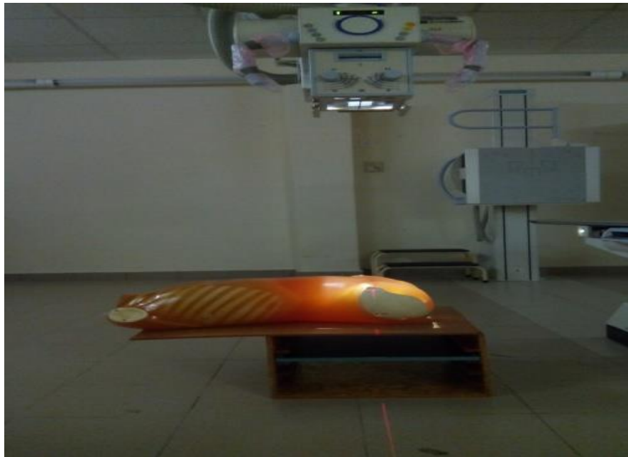
Figure.2: Set-up for the air-gap study of pelvis examination
